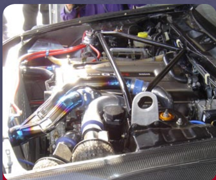
Extensive use of dry carbon and titanium keep weight to a minimum, executed flawlessly on the Powerhouse Amuse Carbon GT-R. Unavailable for Sale
