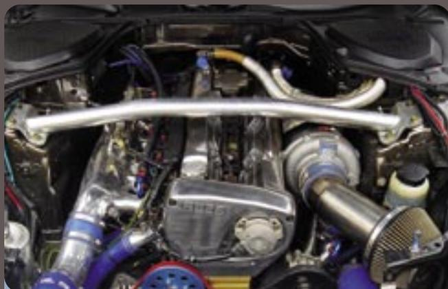
The ORC/Top Secret D1GP Fairlady Z uses the classic RB26DETT to deliver reliable high horsepower while going sideways. Amazingly, Top Secret has installed the RB further back and lower in the engine bay than the stock VQ engine. With excellent weight distribution and over 700hp coming from a mildly tuned RB, expect this Z to do extremely well in the D1GP for 2005. For more information visit [www.oguraclutch.co.jp](http://www.oguraclutch.co.jp).
